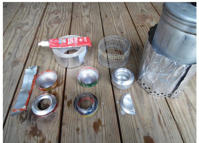
Two old Pepsi-can stoves torn apart to show how they go together, finished stove with pot stand, simmer cap, pot and windscreen.
